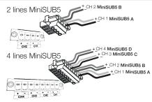
Screw terminal input/link wiring
