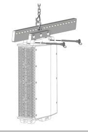
**Pro Tip:** Put one pin in the front first, so you can safely adjust your angle with both hands.
